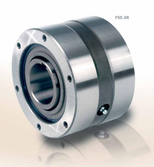
ypes FSO, FSO-GR, and HPI 300 to 700 are sprag type freewheels self-contained, sealed and bearing supported, using two ball bearings.
