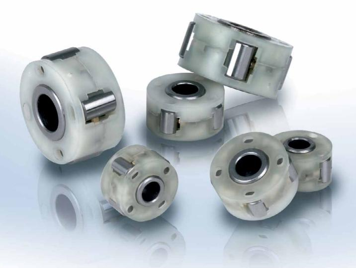
ype KI is a roller type freewheel. It is an assembly comprising of an inner race and rollers fitted into a polyamide cage. This type of unit can not be dismantled. It is designed for small mechanisms in office equipment, or packaging machines, to be mounted inside gears or feed rollers.
