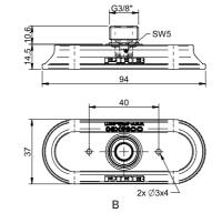
Rubber parts Suction cup 0C35x90P Polyurethane 40 Suction cup 0C35x90P Polyurethane 60
